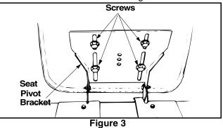
**NOTE:** The seat may have been shipped in a box. Remove the four screws from the bottom of seat and place seat in position against the seat pivot bracket. Follow the directions above to attach the seat.
